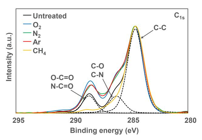
Furthermore, when the C spectrum was separated into waveforms, it was found that the polar groups C–O, C–N, and O–C=O bonds increased in samples treated with O<sub>2</sub>, N<sub>2</sub>, and Ar gases.
