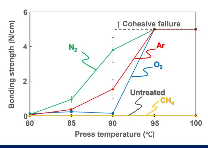
This bond strength increases with the heat press temperature, and we confirmed that the gas species in vacuum plasma surface treatment are effective in the order of  $N_2$ , Ar, and  $O_2$ .
