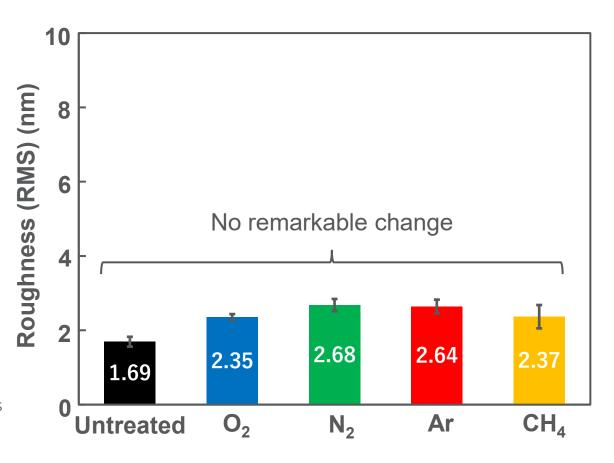
Generally, surface free energy is influenced by physical and chemical properties, but the surface roughness of the samples was similar.
