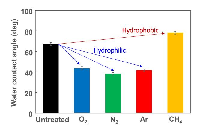
For O<sub>2</sub>, N<sub>2</sub>, and Ar gases, it was confirmed that the PET film surface was hydrophilic. On the other hand, for CH<sub>4</sub> gas, it was found to be hydrophobic.
