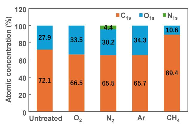
Next, we analyzed the surface composition and found that samples treated with  $O_2$ ,  $N_2$ , and Ar gases had higher oxygen content than untreated samples. In addition, nitrogen was detected in samples treated with  $N_2$  gas.
