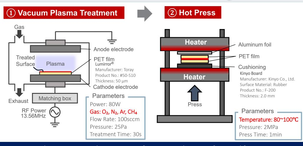
In this experiment, the gas species for vacuum plasma surface modification and hot press temperature were varied.
