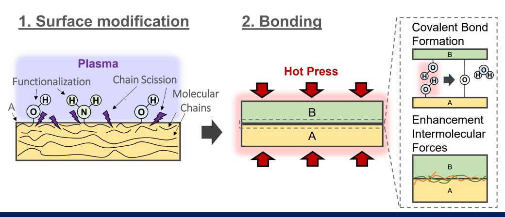
In the case of direct bonding technology using plasma, it has been reported that direct bonding can be achieved by heat pressing after plasma surface modification.
