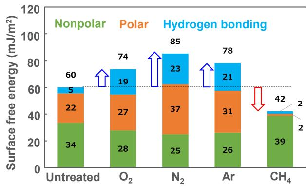
It was found that the surface free energy increased in samples treated with  $O_2$ ,  $N_2$ , and Ar gases, while it decreased in samples treated with  $CH_4$  gas.
